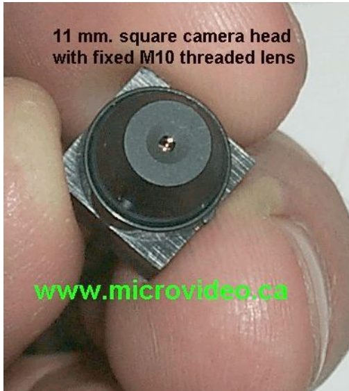
Very small camera heads with Real Japanese CCD chipsets
