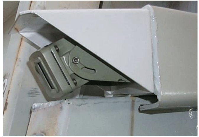
Colour Camera on heavy equipment under weldment
